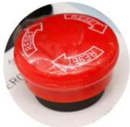
Emergency Stop Button
