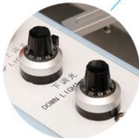
CCD lens light adjust knob
